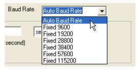
you must set the baud rate in the opening connection menu of the Global Logger II software to this speed, or the logger will not communicate.
