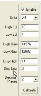
High EU: The High EU field is the engineering unit where the highest output from the sensor is achieved during the calibration process, in this case a pH of 10.
